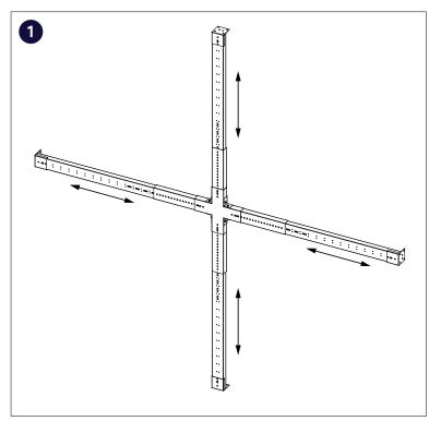
The TUISKU-AK installation frame is designed to make installing the multielement TUISKU pieces easier. The dimensions of the installation frame are adjustable to fit the opening.
