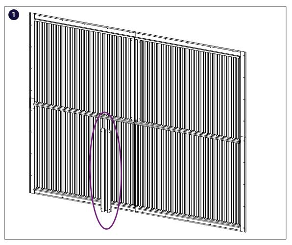
1 The whole is finished by attaching the cover strips that come with the delivery to the front.
