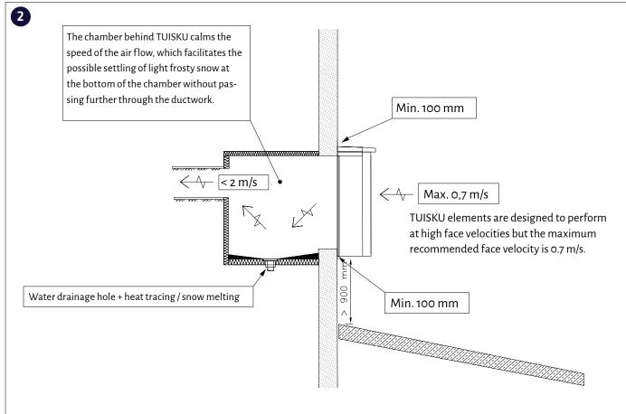
It is advisable to build a chamber and drainage similar to the figure behind the snow covers to prevent light snow and water caused by exceptionally strong winds from getting into the ducts.
