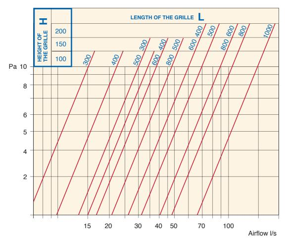
The sound level is less than 25 dB(A), when pressure drop is less than 20 Pa. Recommended pressure drop max 15 Pa
