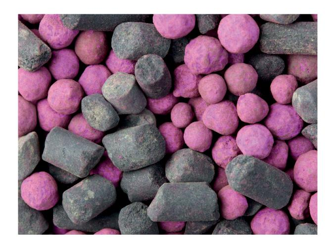
CEKP 8 is a mixed filter medium combining the best properties of activated aluminum oxide and activated carbon.
